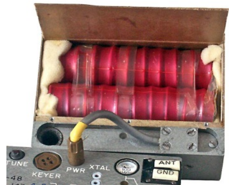
Battery BS-48 with cover opened showing two rows of NiCad cells. When not in use the power cable was stowed into a round compartment on the left.
